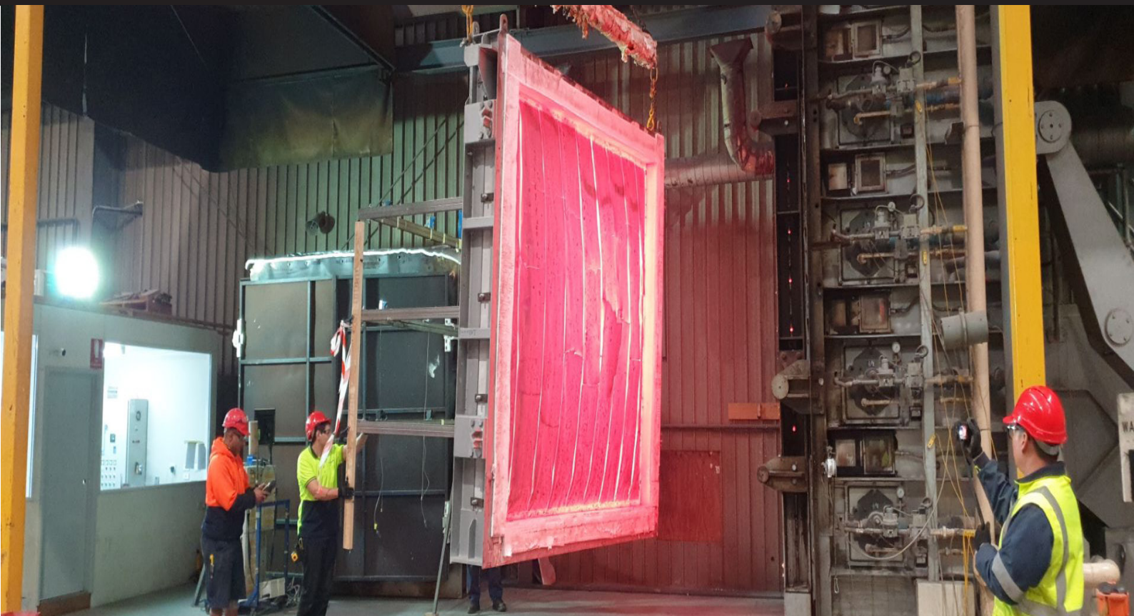
K8 SUPAPANEL® wall testing after a 4 hour fire test carried out by Warrington Fire Testing & Certification
